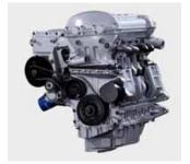
the compression ratio. The SVC engine can be run at the optimum compression ratio of 14:1 at low load and lowered to 8:1 at high load with supercharging (225hp, 224 lb.-ft./1.6L). This concept reduces fuel consumption by up to 30% when compared to a larger conventional NA engine of similar power output. (http://www.saabnet.com)
