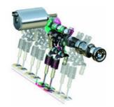
does not need specific fuel grades or fuel qualities because of its fine atomization of fuel. (http://www.bmwworld.com)
