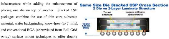
the memory capacity for increased device functionality while allowing manufacturers to maintain size reduction roadmaps. This technology allows for very efficient use of mother-board real estate, reducing size and weight and supporting the customer's system level cost reduction needs. Stacked CSPs also offer the user the flexibility of combining custom memory with off-the-shelf devices to further reduce total systems cost. (http://www.amkor.com)
