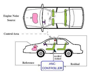
Technology) research lab had applied ANC system to noise suppression on vehicle. It can reduce use of sound insulation material. (<a href="http://ultrapark.kaist.ac.kr">http://ultrapark.kaist.ac.kr</a>)
