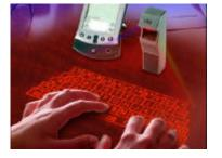
component size, simple processing, high accuracy and ease of use. All that is necessary to use the keyboard is a flat surface. (<a href="http://www.vkb.co.il">http://www.vkb.co.il</a>)
